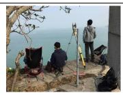
Land-Based Theodolite Tracking Survey for CWD at Lung Kwu Chau
