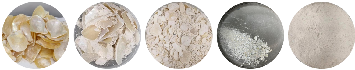
Pearl shell from raw material to final nano-particle
