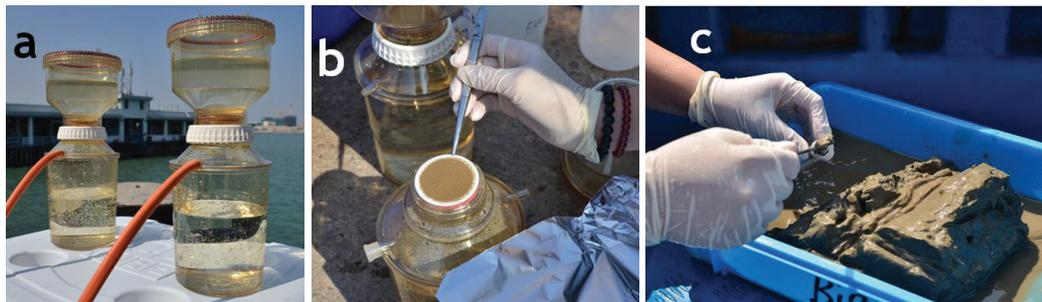
**Fig. 4** **a** Photo showing filtration of seawater samples. **b** Photo showing collection of the filter after the filtration using commercial aluminium foil and forcep. **c** Photo showing collection of the sediment samples using sterile 15ml centrifuge tube and spatula.
