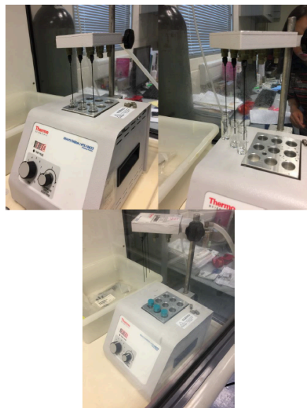
Fig 7. Sample hydrolysates drying under nitrogen stream
