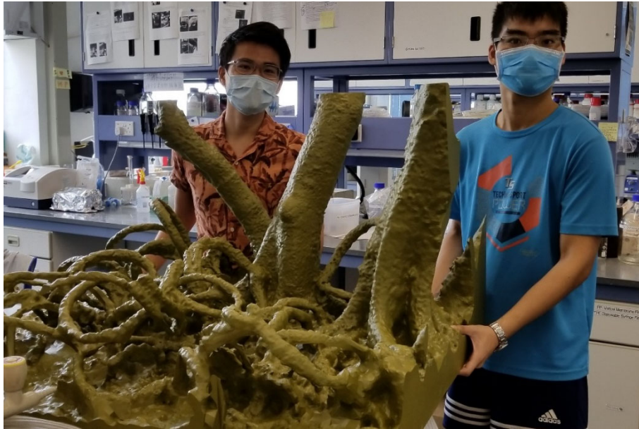
Figure 8. The first printed 3-D model. The model measures 1x0.9x0.7 m in size and is coated with a low-volatility paint to match the natural colour of the tree.
