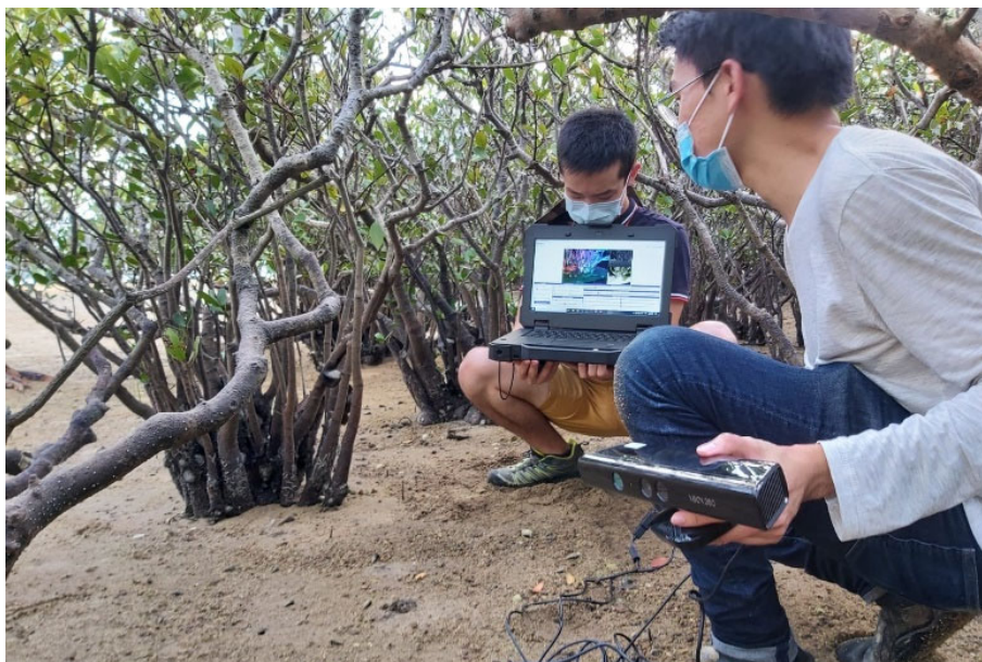
Figure 2. Research assistant Rinaldi Gotama (right) and student helper Vincent Tran (left) scanning an Aegiceras corniculatum patch using a Kinect V1. The Kinect was plugged to a waterproof laptop computer, which showed the scanning process in real time.
