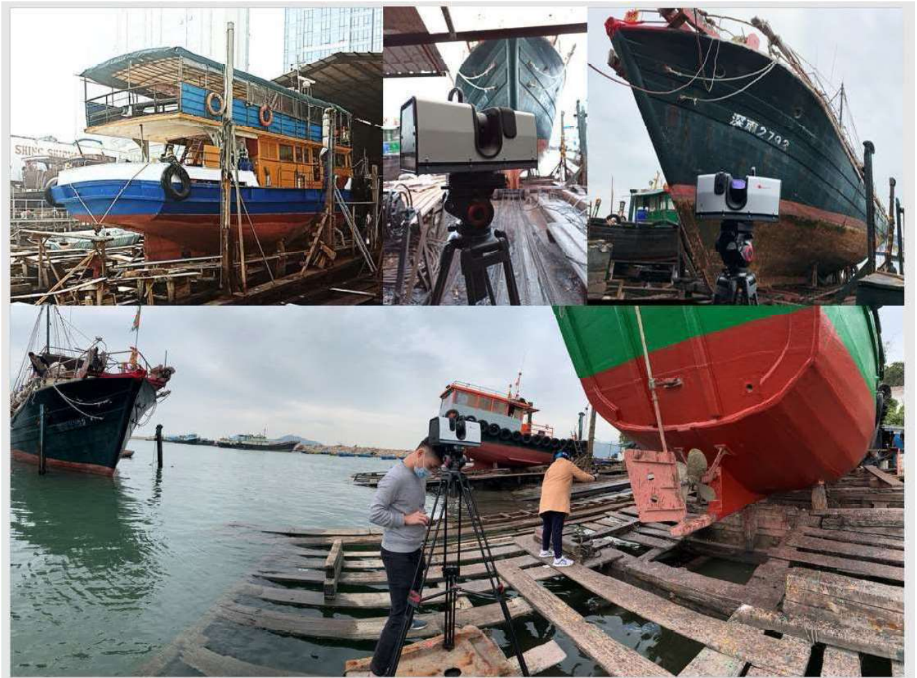
Fig. 7. Vessels scanned with the long-range 3-D scanner in boatyard in Ap Lei Chau.
