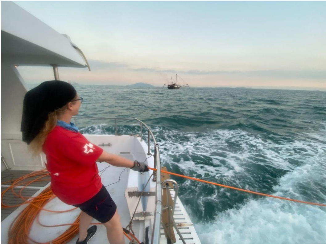
Figure 3. The cabled hydrophone array ( Seiche , United Kingdom) being deployed from the research vessel near the Soko Islands. An active illegal trawler operating in Hong Kong waters can be seen in the background.
