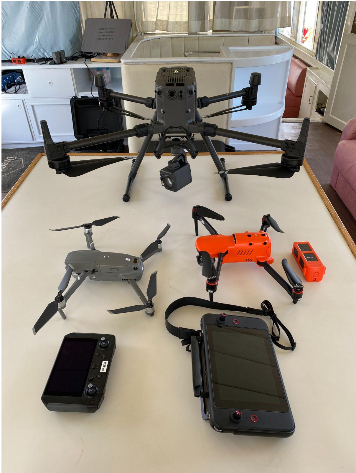
Figure 5. The Unmanned Aerial Vehicles (UAV) used during systematic surveys: DJI Matrice RTK 300 (top), DJI Mavic 2 Pro (left) and an Autel Evo II (right). Not pictured: DJI Mavic 2 Enterprise.
