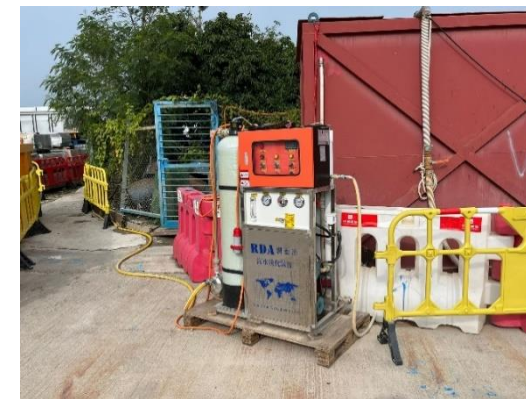
Use of Seawater Desalination Reverse Osmosis System to generate freshwater for water spraying to reduce generation of fugitive dust
