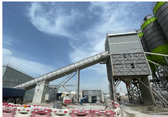
Fully enclosed conveyor belt and mixing tower for concrete batching
