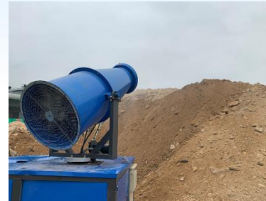
Dust suppression – use of automated mist sprayers & sprinklers
