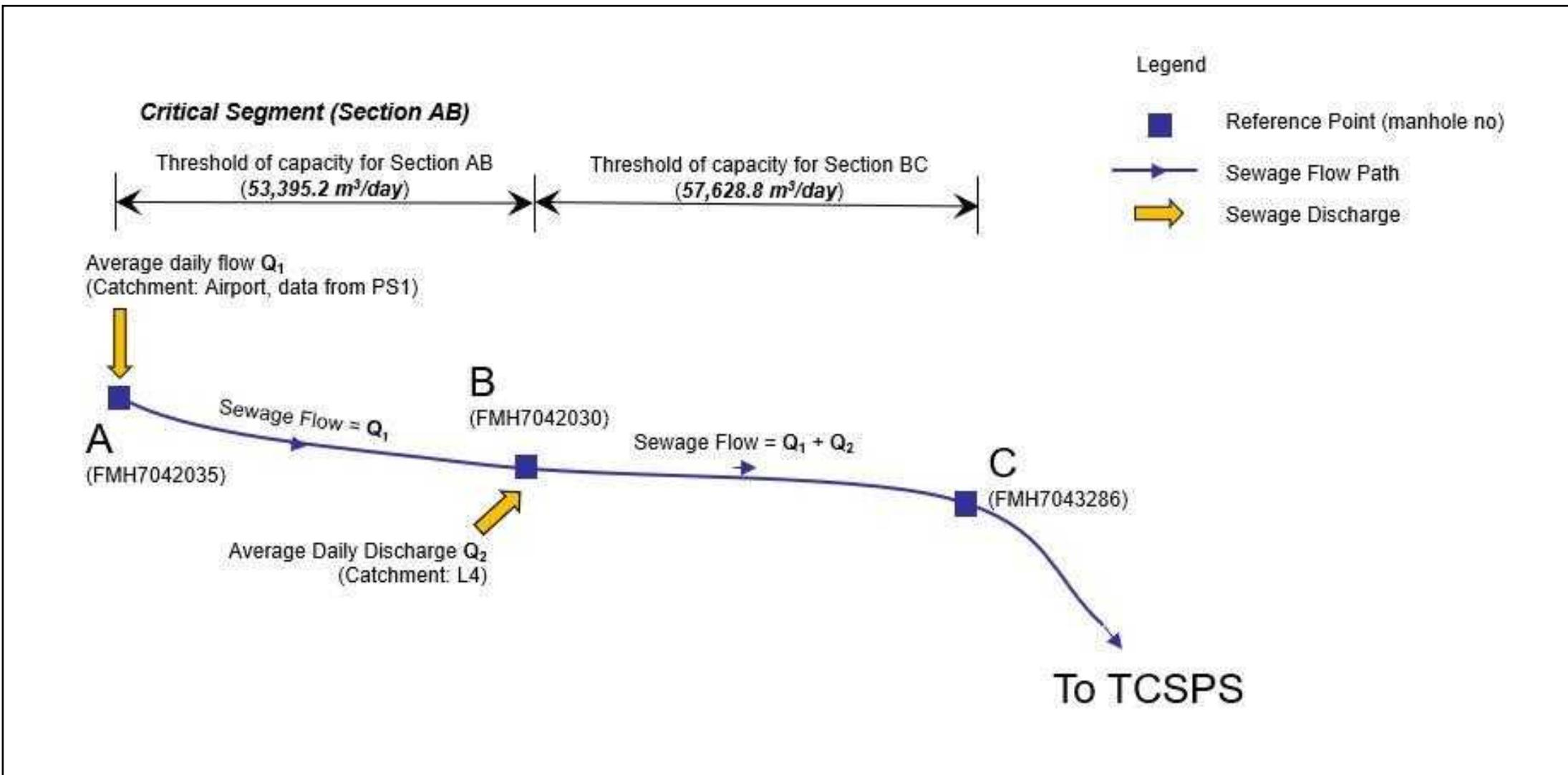
FIGURE 2.8 SCHEMATIC DIAGRAM FOR SEWERAGE SYSTEM FLOW MONITORING
