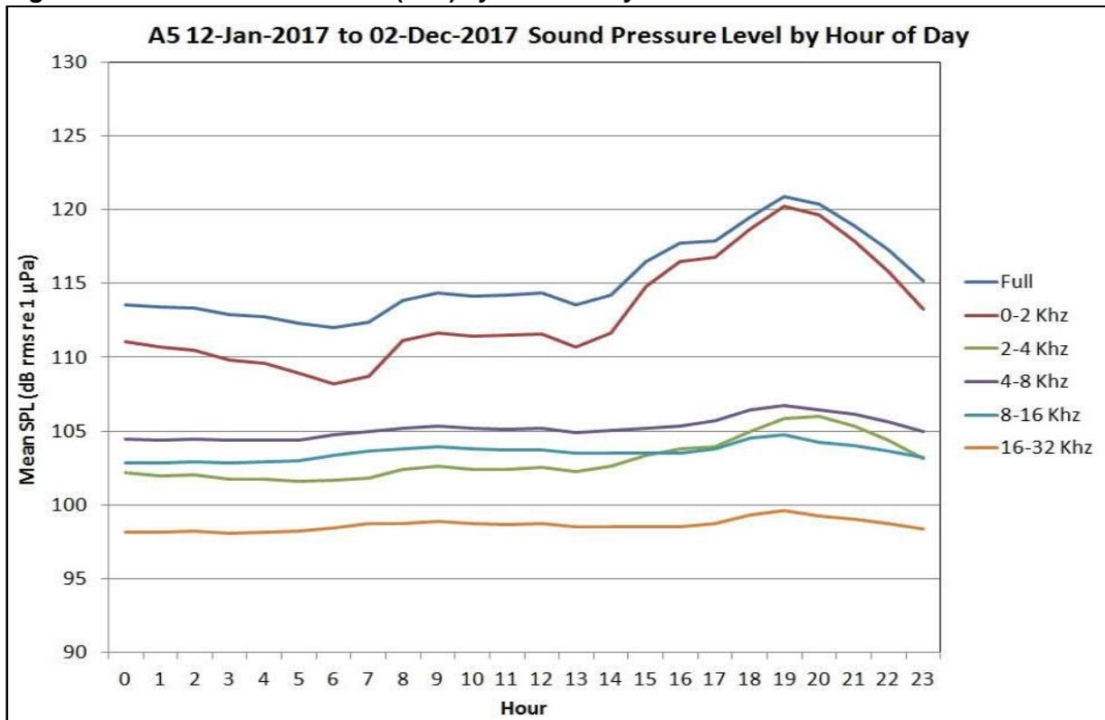
Figure 30: Sound Pressure Level (SPL) by Hour of Day and Solar Season recorded in 2017
