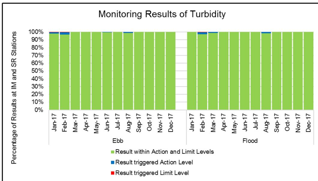
During the reporting period, 0.5% of the turbidity monitoring results triggered the corresponding Action or Limit Level. Due to the small number of results triggering the Action or Limit Level, and the relevant investigation findings presented in the Construction Phase Monthly EM&A Reports, it is considered that the Project did not cause adverse impact on turbidity level at all water quality sensitive receivers.
