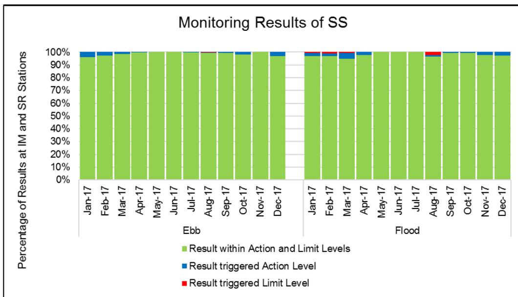
During the reporting period, 1.6% of the SS monitoring results triggered the corresponding Action or Limit Level. Due to the small number of results triggering the Action or Limit Level, and the relevant investigation findings presented in the Construction Phase Monthly EM&A Reports, it is considered that the Project did not cause adverse impact on SS level at all water quality sensitive receivers.
