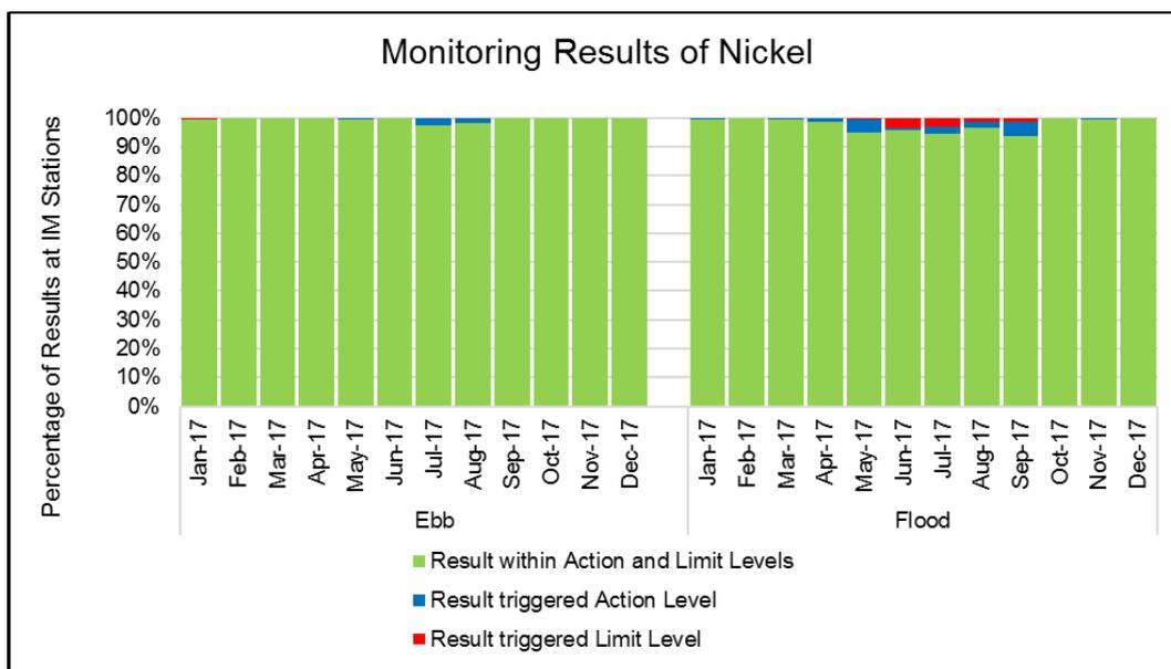
During the reporting period, 1.2% of the nickel monitoring results triggered the corresponding Action or Limit Level. From the graph, it is noted that the majority of cases were recorded in the wet season during mid-flood tide, which might suggest the existence of a seasonal, tide-specific effect that could have led to episodes of relatively high nickel concentrations, and is not related to the Project activities.
