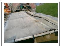
Dump Truck with Mechanical Truck Cover Adopted by Contractor for Delivering Dusty Waste Material
