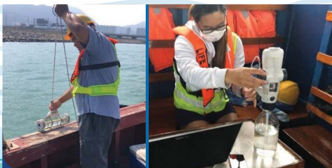
定期進行一般及深層水泥拌合法工程的水質監測，以檢查是否符合《更新環境監察及審核手冊》中的監測參數 General and DCM-specific water quality monitoring is conducted regularly to check the compliance of parameters as stated in the Updated Environmental Monitoring and Audit Manual
