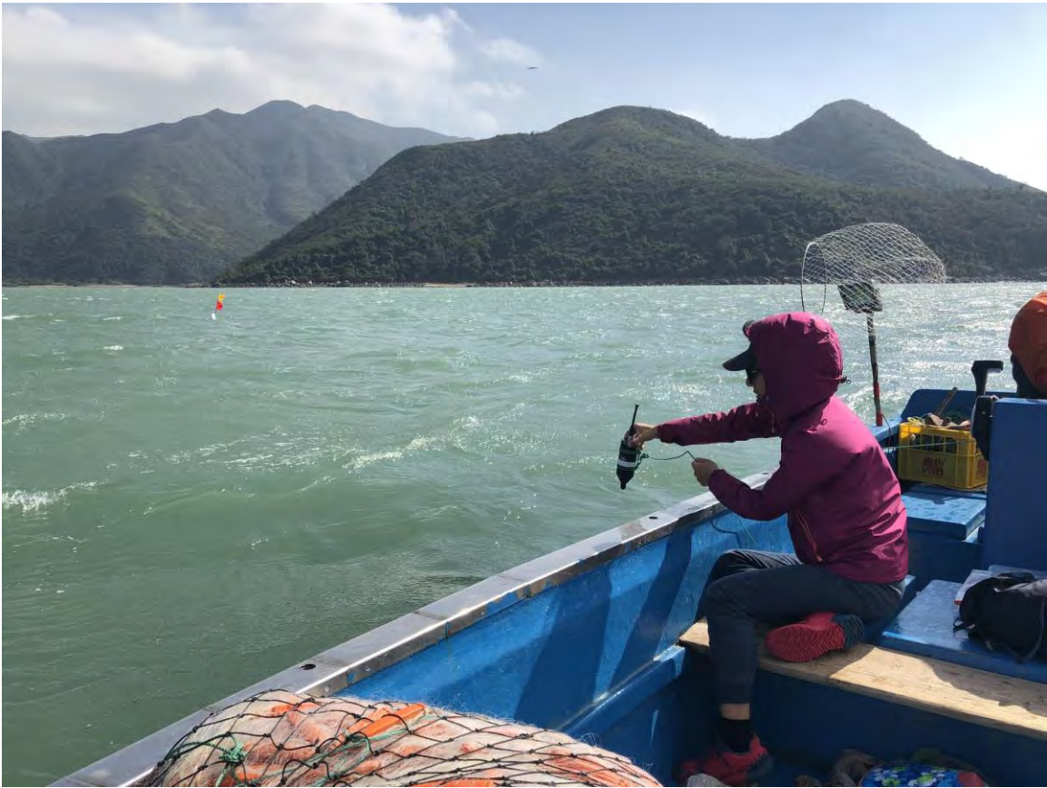
Figure 4. An AAD being deployed near a gillnet at Yi O, Lantau, during a dedicated survey
