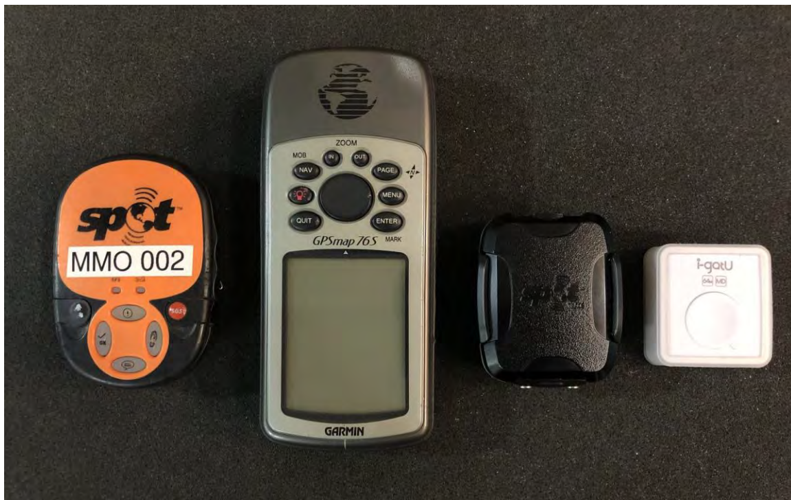
Figure 13. The tracking devices trialled between April and December 2018 (from left to right): a SPOT Satellite GPS Messenger, a Garmin GPS map 76S, a SPOT Trace and an iGotU ST-600.
