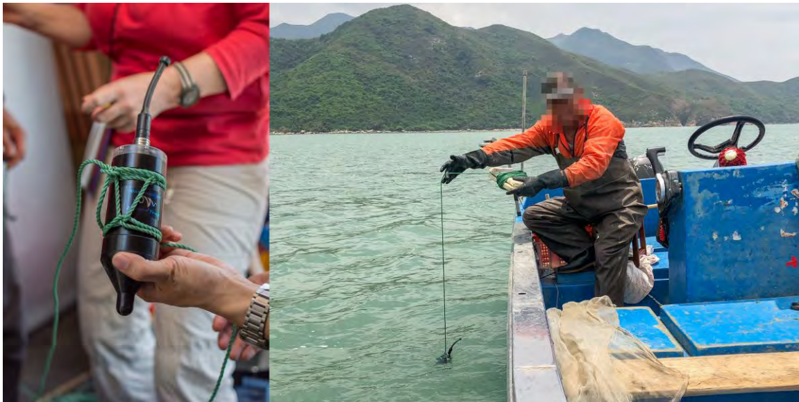
Figure 2. The fisherman demonstrating the attachment of the AAD (SoundTrap) to floats with nylon rope (left) before being deployed with on a gillnet (right).
