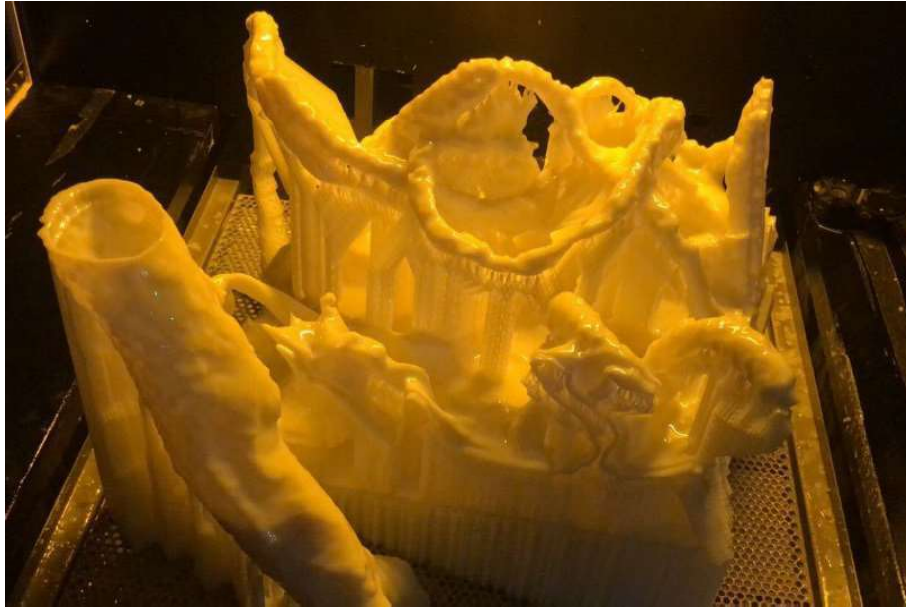
Figure 6. 3D printing process of a mangrove tree model using synthetic resin. Due to its large size, the model was printed in several separate pieces and glued together.
