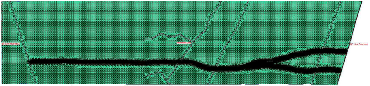
Figure 23. Mesh of the 2D Flow Area. The geometry was created with HEC-RAS Mapper. The tidal channel is shown almost in black as a consequence of the high-resolution refinement region (2 m x 2 m grid size) that was chosen to represent the more complex channel hydrology.
