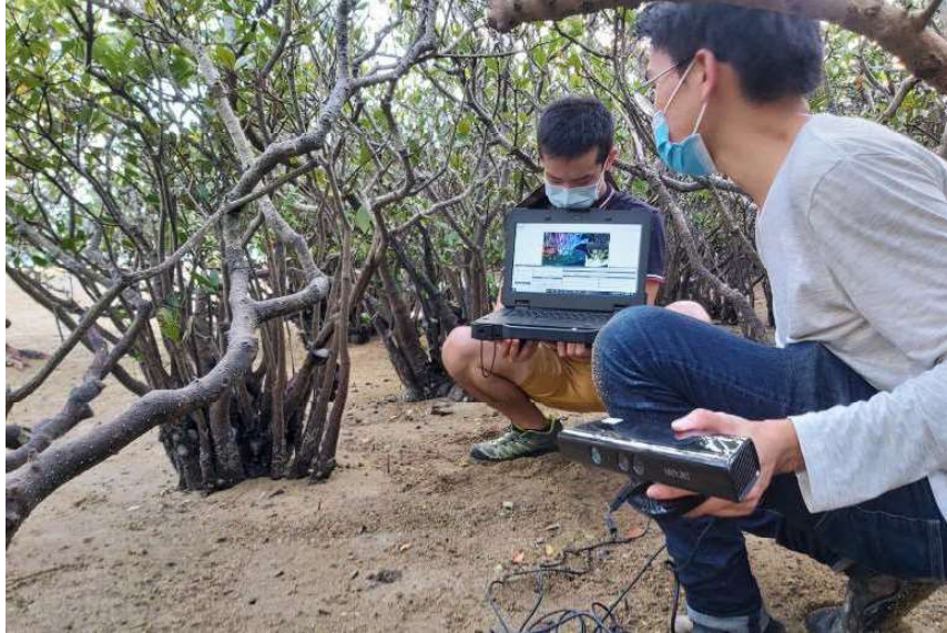
Figure 4. The Xbox Kinect sensor. Project members scanning an Aegiceras corniculatum patch using a Kinect sensor. The sensor was plugged to a waterproof laptop computer, which showed the scanning process in real-time.
