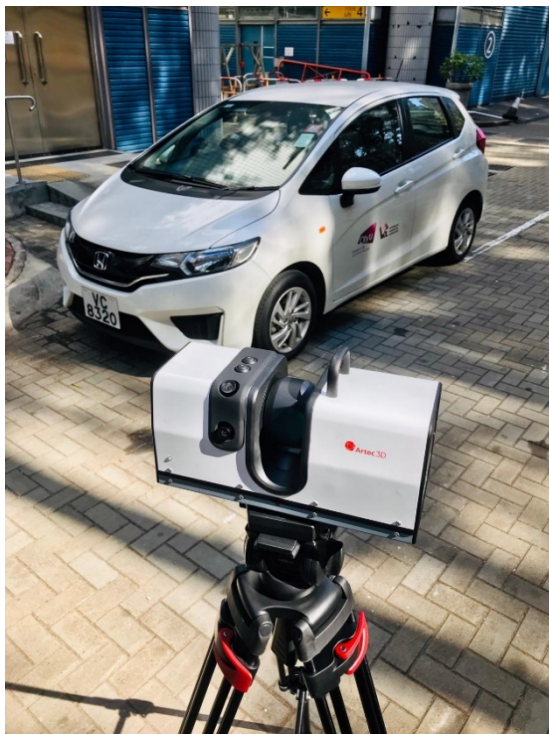
Fig. 8. A trial application of 3DSS on a car scanned by our team in City University of Hong Kong using Artec Ray. This equipment and scanning technique will be used to document and describe the types of suspected trauma-inflicting instrument using 3DSS technique, leading to injury induced by vessel interaction in stranded cetaceans.
