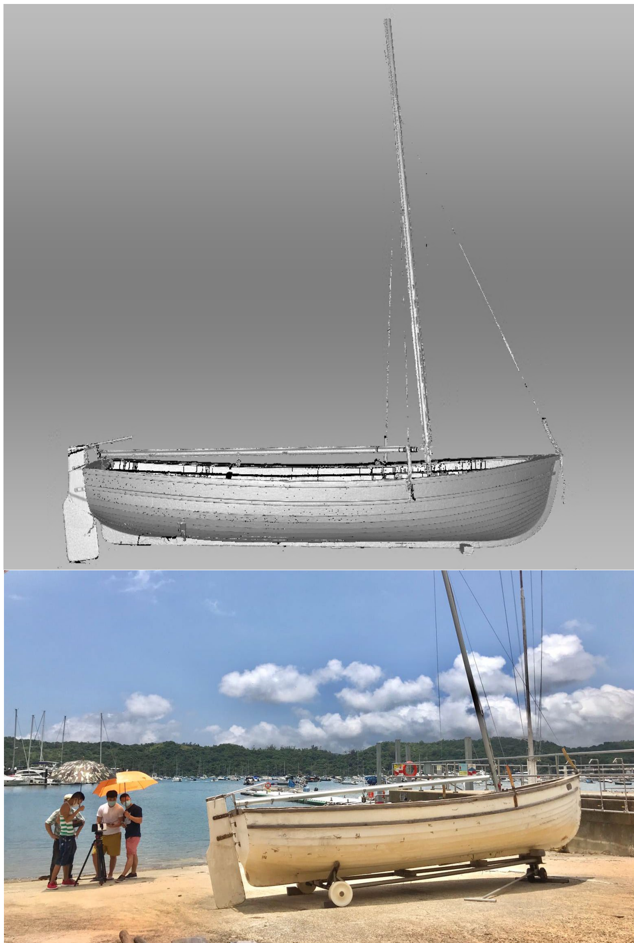
Fig. 10. A demonstration of the 3DSS reconstructed model (upper) and the original marine vessel (bottom) scanned by our team using Artec Ray in May 2020.
