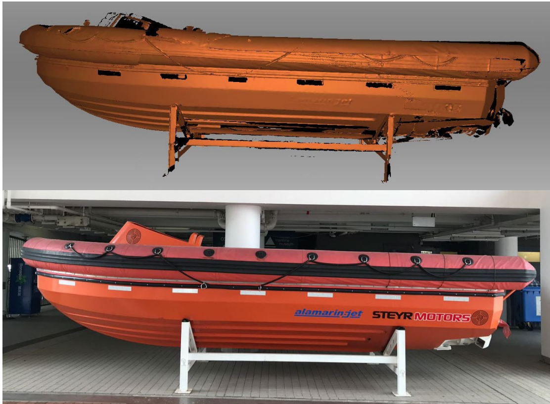
Fig. 9. A demonstration of the 3DSS reconstructed model (upper) and the original marine vessel (bottom) scanned by our team using Artec Ray in May 2020.
