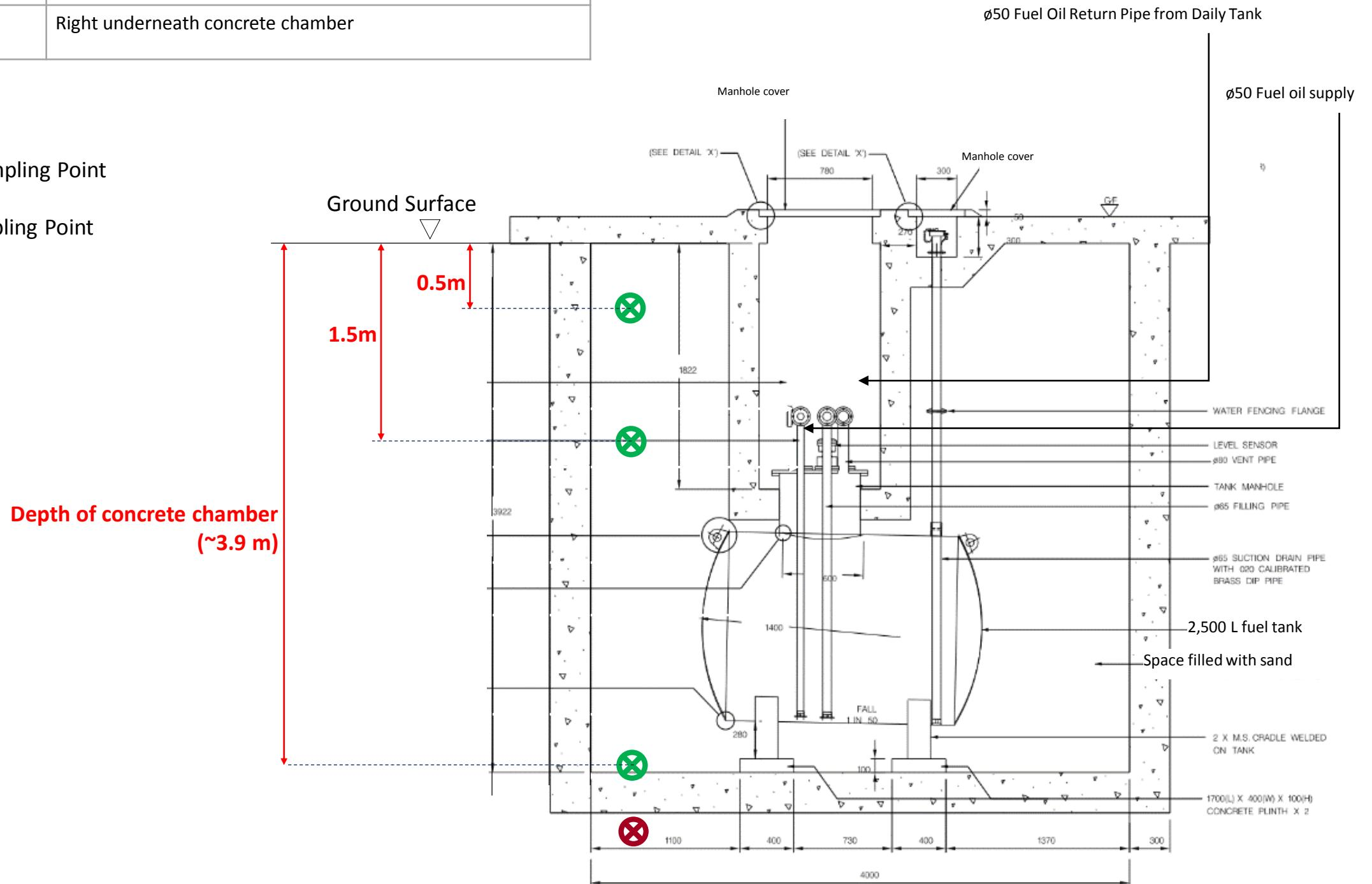
Indicative Sampling Point Selection of 2,500 L Underground Fuel Tank of Emergency Power Supply System No.1 (i.e. **BH1**)
