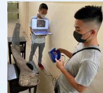
3D surface scanning of cetacean specimens
