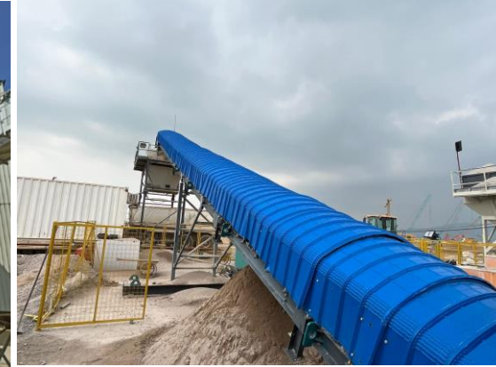
Conveyor belts were fully enclosed to prevent fugitive dust emission
