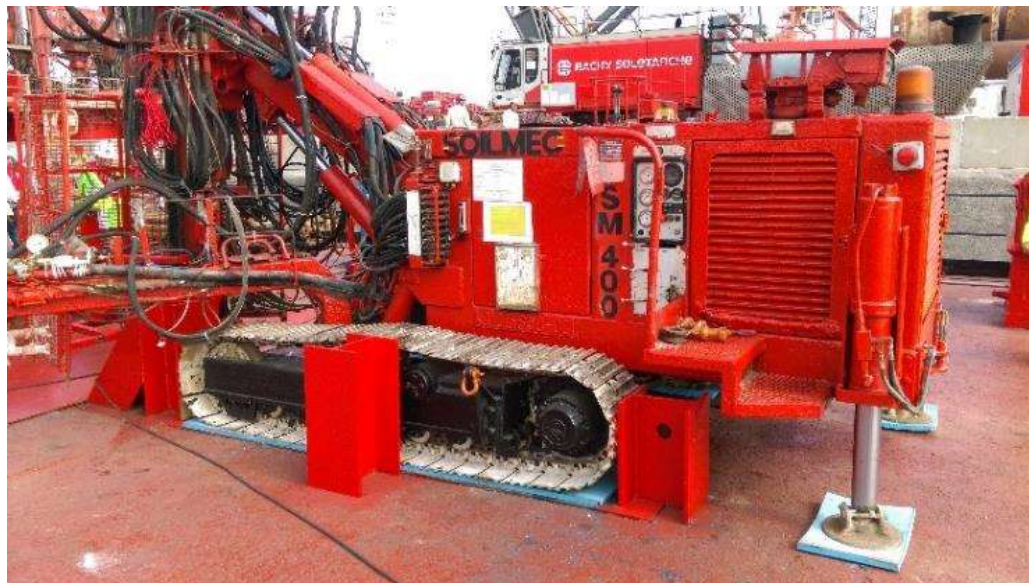
Isolation pads placed under noisy equipment to mitigate ecological impacts
