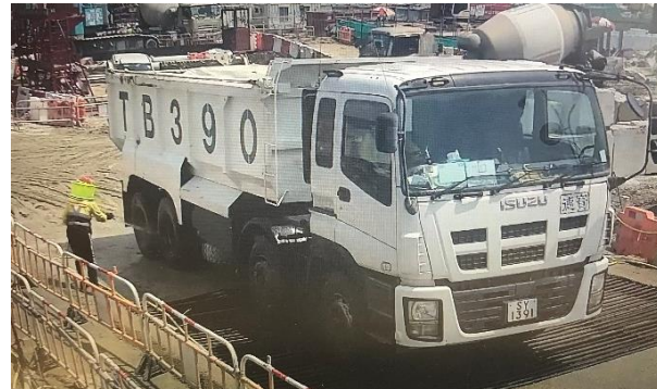
Images showing the body and wheels of the dump truck were properly washed and loadings were covered before leaving the site
